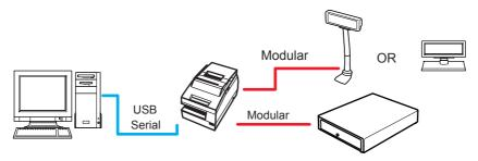
The Y-connection is a connection method to connect the computer and the Customer Display via the TM printer.
